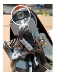
4) Carefully slide Fuser Belt toward the front (wire side) of the assembly to remove.
