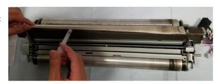
Optional – Remove large Steering Roll Spring to make Fuser Belt installation easier.
