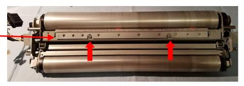
7) Gently roll fuser over. Loosen two (2) screws and remove lower wick.
