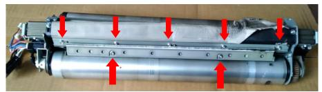
8) Install new Sheet (be careful not to fold or scratch sheet surface) and Sheet Plate with the beveled corner toward the rear (gear side).
