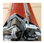
3) Orient the Fuser Belt Assembly as shown. Press down on the spring loaded Steering Roll and insert an M4 screw as shown to relieve the belt tension.
