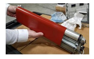
5) Clean any oil and dirt residue from all visible surfaces and inside belt.
